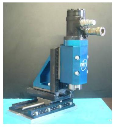
Utilising the same design concepts as the SJP Series the KCM Compact Mill is designed to get into small tight spaces. At just 350mm Wide, 350mm Deep, 500mm High (less with RA Drive Motor) the KCM Compact Milling Machine is compact & versatile.
