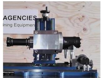
This feature provides the operator with the ability to machine a surface other than the surface below the milling machine including directly above.
