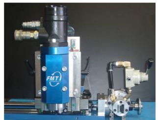
Our custom designed gearbox & clutch assembly allows the operator to easily engage or disengage the drive as required improving setup time while still providing accurate adjustment. In addition to this, changing feed rate or from pneumatic to hydraulic feed is quick & easy operation.
