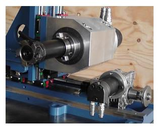
Another important feature of the SJP Portable Milling Machine is the ability to reposition the XY AXIS assembly in relation to the X Axis
