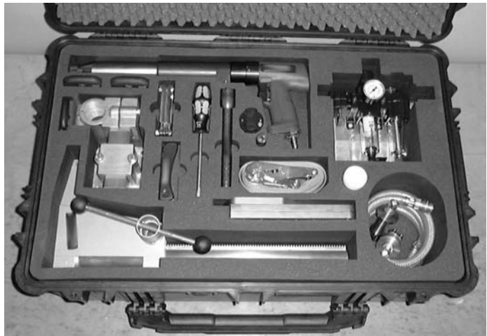
Globe valve extension kit with pneumatic motor (standard kit does not include maintenance unit)
