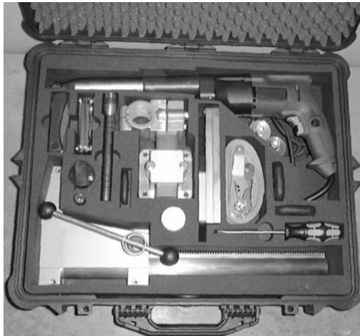
Globe valve extension kit with electric motor
