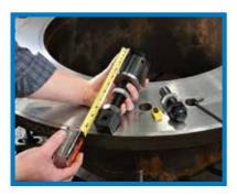
Extend feet into flange. Indicate, level and tighten leveling feet and stationary feet.
