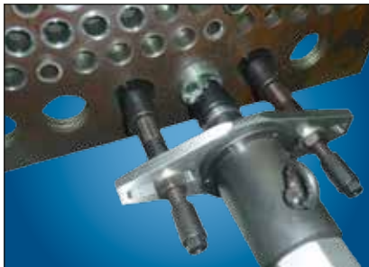
⌘ Reducing tube wall on a 6" thick tube sheet prior to punching.
