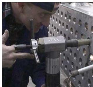
Operator trimming back tubes prior to seal welding
