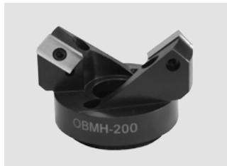
Custom, precisely designed head. Dedicated for outside bevelling of both tubes and pipes. Sized per tube or pipe diameter and angle of required weld bevel. The heads are precisely engineered so that the inserts cannot damage the shaft or locking jaws.
