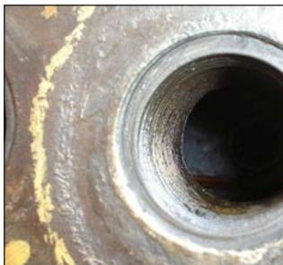
Plug hole before re machining the gasket seat
