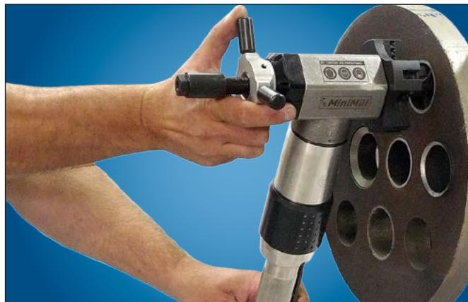
Facing, bevelling tubes quickly and safely.
