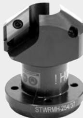
Custom designed head dedicated for strength weld removal. The heads are sized per tube diameter and are precisely engineered so that the inserts cannot damage the shaft or locking jaws. Simple, trouble-free set up makes these heads very advantageous.
