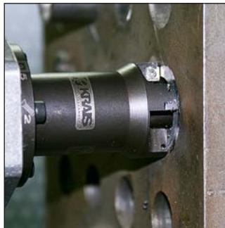
☛ A seal weld removal head with carbide inserts.
