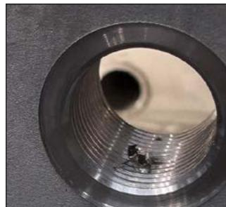
All types of water box materials can be machined with the carbide inserts of the MiniMill 300 GFF.
