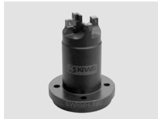
Size specific heads designed for removing seal welds from tubes. Suitable for weld removal on carbon, duplex, inconel and other exotic alloys. Utilizes 4 sided carbide inserts.
