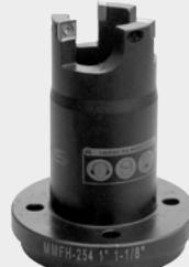
A tube facing milling head suitable for machining tubes manufactured from very hard materials such as duplex, inconel and other exotic alloys. Utilizes 4 sided carbide inserts.
