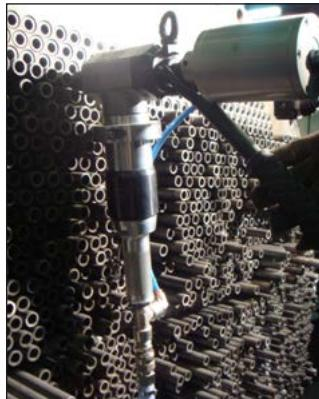
☞ A real application where a customer is shortening a bundle. MiniMill can deal with this task quickly and efficiently.
