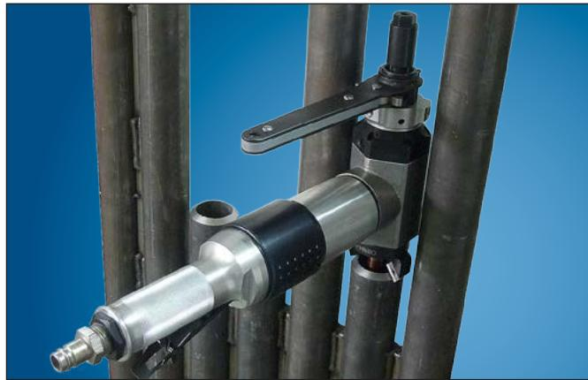
❖ Fitted with our optional multi feed system, the Mini Mill is easily changed from it's star wheel configuration to a ratchet drive for fast and accurate preps on water wall panels.
