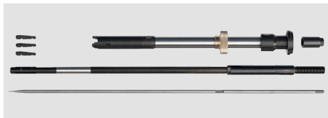
Special attachment for facing tubes in fin fan gas coolers. A locking shaft with adjustable length and a support bushing are screwed into the plug thread, making this tool the best one available on the market today. The cycle is approx. 1 min from tube to tube. For this application we recommend our 300 rpm machine
