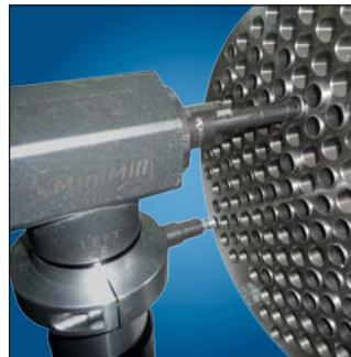
☛ Micro shaft trimming of 5/8" stainless tubing.
