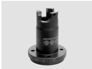
A tube facing milling head suitable for machining tubes manufactured from very hard materials such as duplex, inconel and other exotic alloys. Utilizes 4-sided carbide inserts.
