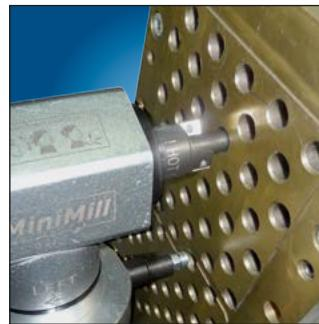
☛ 14 x 1mm tubing being trimmed back quickly and efficiently.
